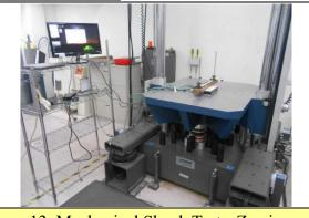
13. Mechanical Shock Test: -Z axis
