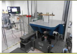
Mechanical Shock Test: -X axis
