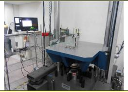
10. Mechanical Shock Test: +Y axis
