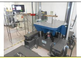
Mechanical Shock Test: +X axis
